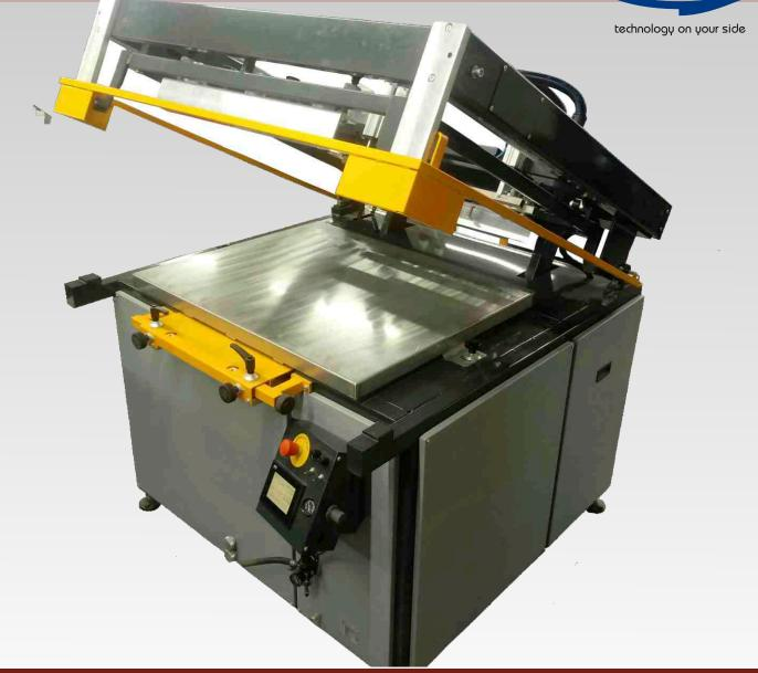
FARGO is flatbed machine with angle lifted print head. Screen lifting and carriage drive made with moto-reducer driven by frequency converter.
